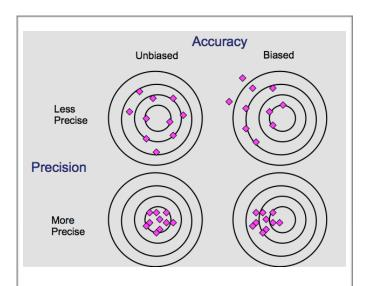
**Difference between** *Accuracy* and *Precision.* Precision refers to how similar replicate samples are to one another. Accuracy refers to how similar replicates are to some true value. You might have a very expensive balance that weighs to the nearest 0.0001g but which is always 10 g too heavy. In this case the expensive balance is precise but not very accurate.
